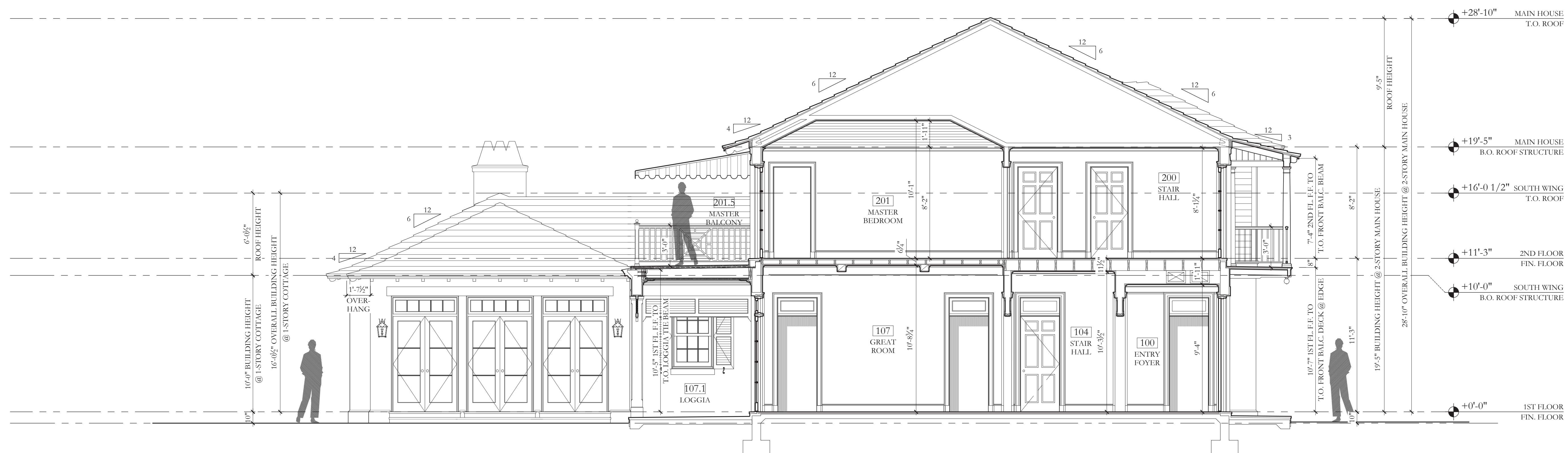
1 BUILDING SECTION, LOOKING WEST 1/4"=1'-0"
