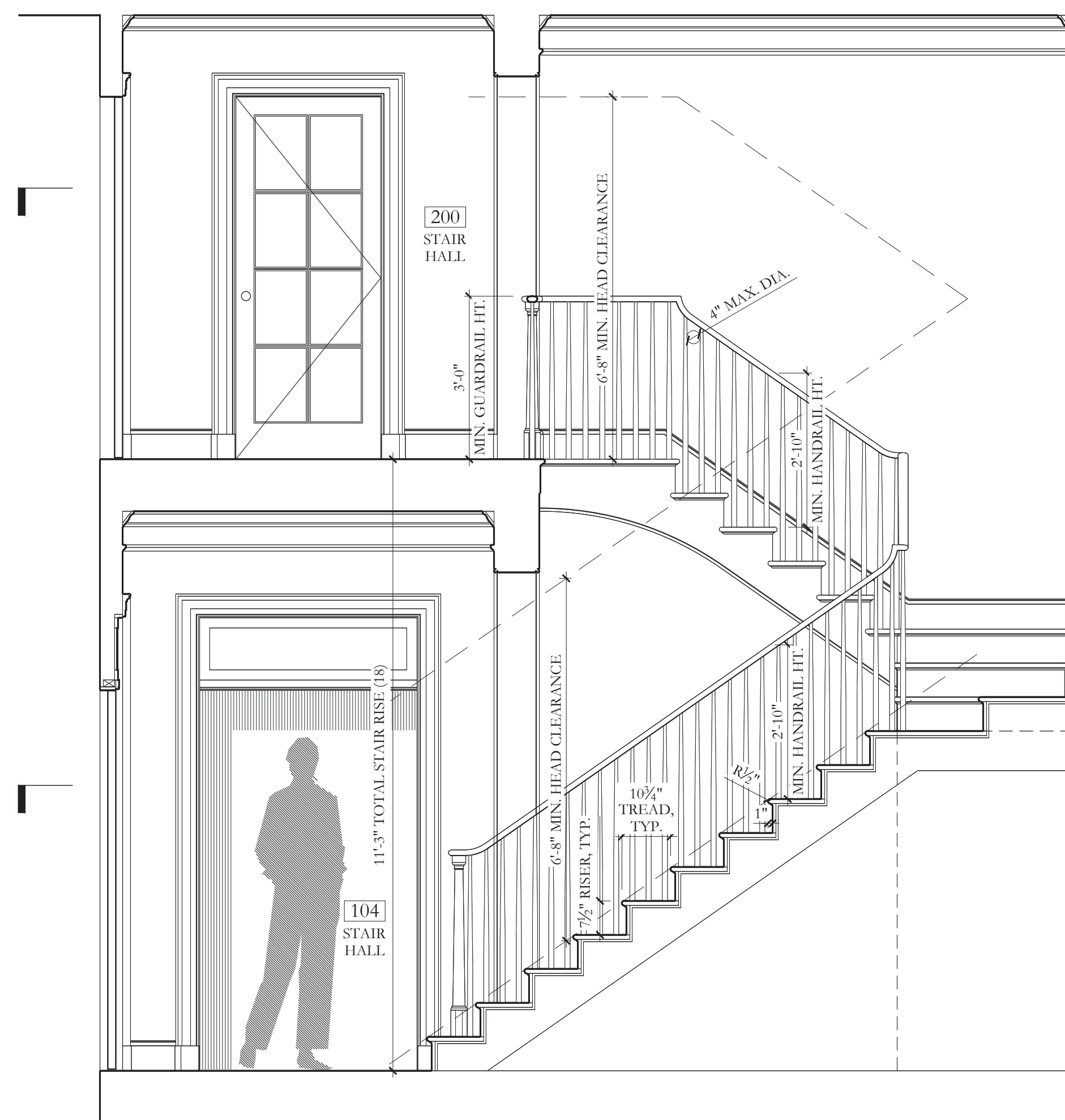
2 104/200 STAIR HALL SECTION, LOOKING NORTH 1/2"=1'-0"
